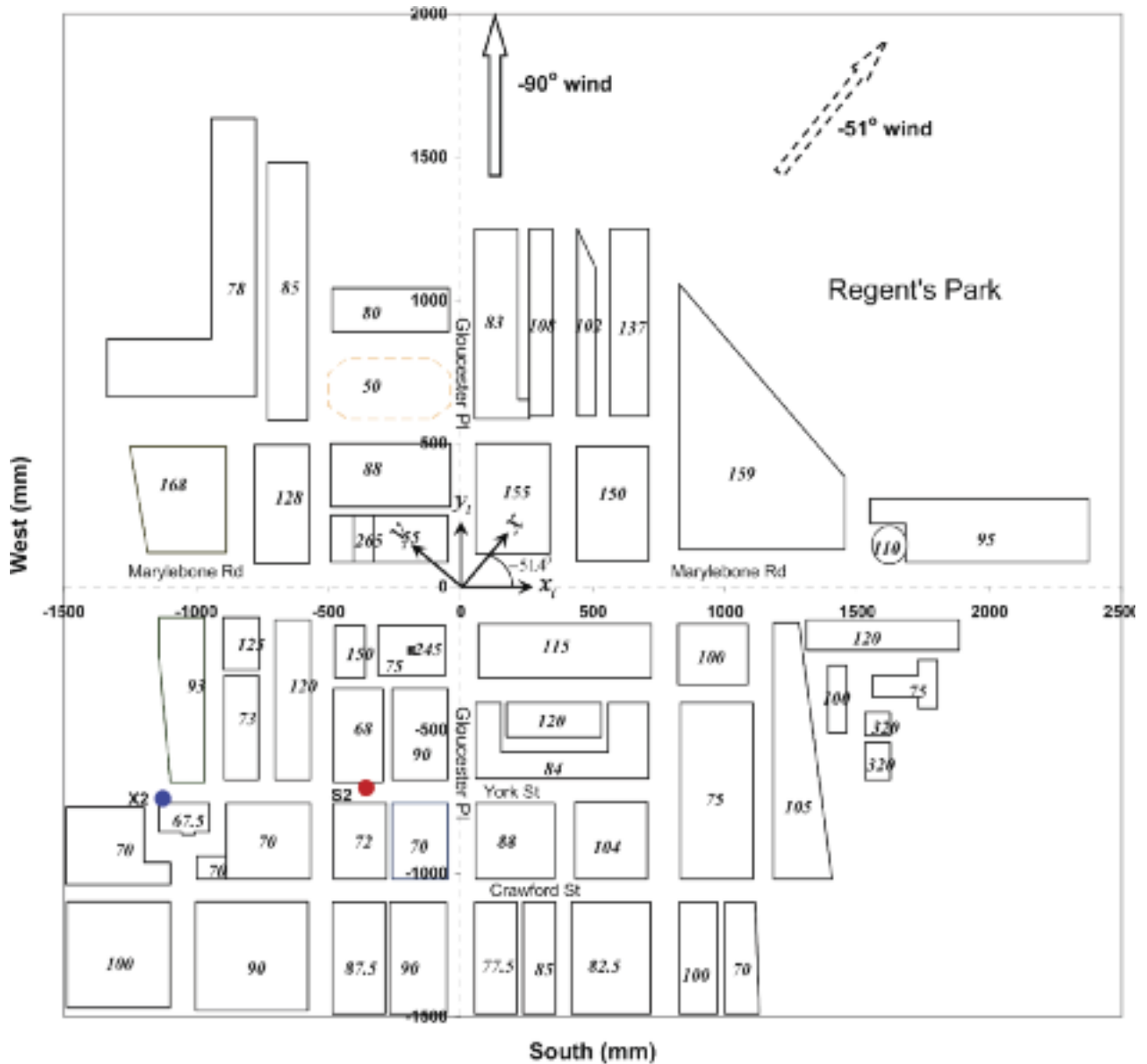
Figure 7: Plan view of the 1:200 wind tunnel model of the DAPPLE site. Numbers in italics on each building block indicate its height in mm; the model coordinates are marked in mm, with x_1 from west to east, y_1 from south to north and z from ground to top respectively; x , y , z are the computational coordinates (see Figure 8).
