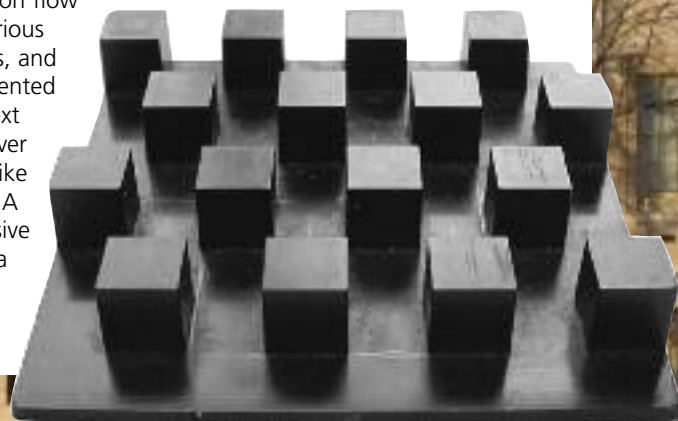
Figure 1: A view of one of the repeating units used in the experiments [4]. The oncoming flow is from top to bottom
