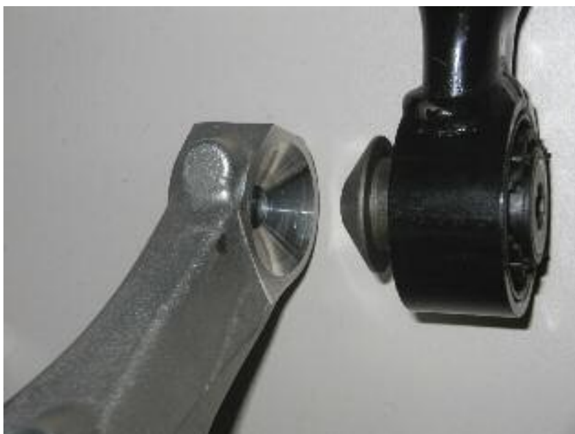
Figure 1: Close-up view of Knuckle Cone Seat and Inner-Sleeve
