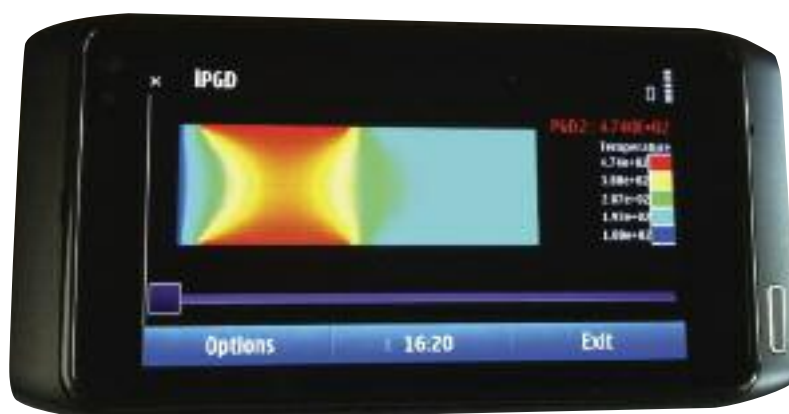
Figure 2. The PGD-based application is able to determine the optimum values for working temperatures in the pultrusion furnace and provides a color map of the temperature field. In the event of malfunctioning values (a heater is broken, for instance), thermocouples will send a signal to the phone to indicate that they are registering non-optimal temperatures. The following step, determines which heater is not working well, by solving, always in real-time, the corresponding inverse problem. Once it is identified, the working temperature of the “healthy” heaters should be optimized again (bottom left figure) to allow the furnace to continue working in the presence of a broken heater. The resulting optimized temperature field in the case of one malfunctioning heater is shown in the bottom right figure.
